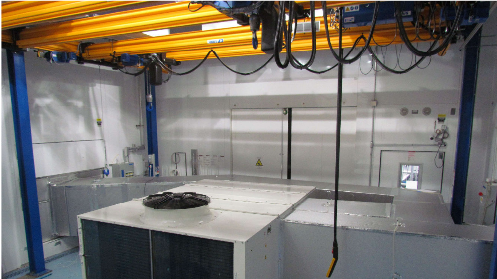
40kW Rooftop UUT ready for capacity testing
