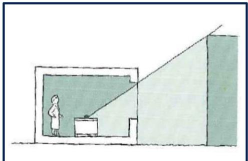
Sunlight diffused through openings is considered direct and reflected by surfaces and/or walls is considered indirect
