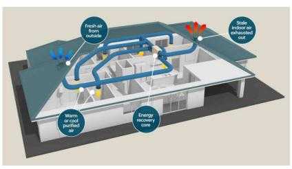
2.It features a heat exchanger combined with a ventilation system for providing controlled ventilation into a building. By way of two fans, ERVs draw clean, fresh air into a home or office and remove stale air.
