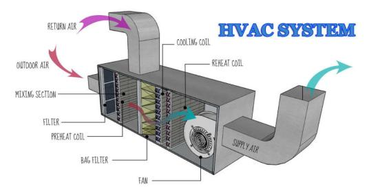
Mechanical HVAC systems are the most prevalent approach to conditioning modern buildings. While often scorned for their energy consumption, well-designed mechanical systems can be very energy efficient.
